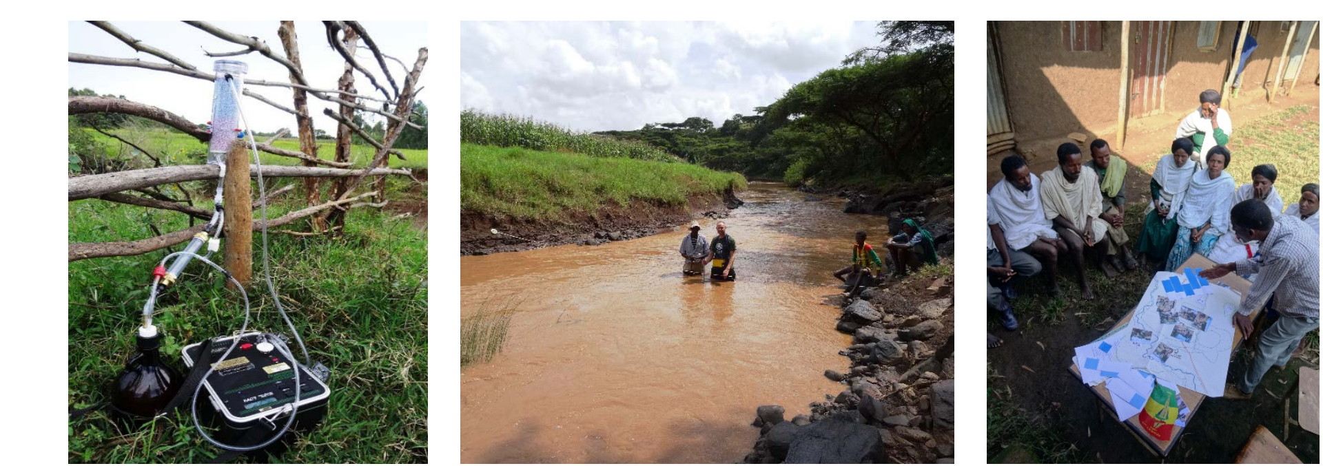
Measuring radon-222 concentration (left), flow-gauging in the Kilti river (centre) and a workshop with the Dangesheta local community
