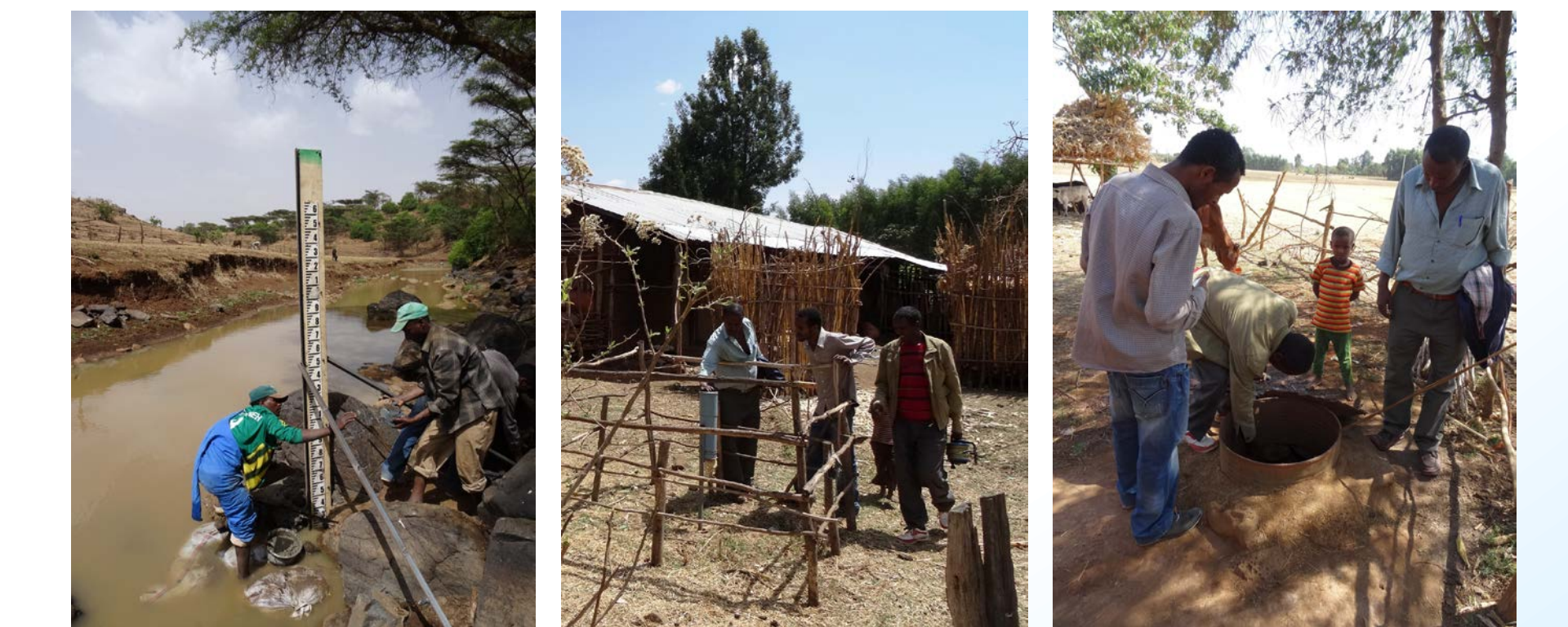
Reconstruction of the Kilti river gauge board (left) following damage during wet season floods, the rain gauge (centre) and measuring depth to groundwater in a monitoring well
